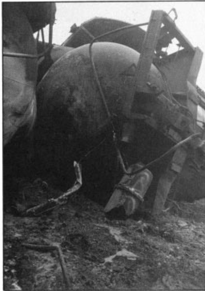
Figure 6.—Tank car ACFX 84070 in derailment pileup
