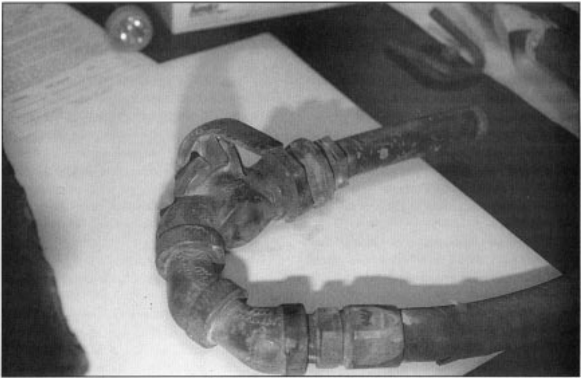
Figure 8.--Angle cock of flat car ATSF 92018
